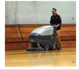
After the entire floor is dry-scrubbed, rinse the entire floor. Use the autoscrubber equipped with a worn set of SPP pads and WAXIE Ultra Clean Wood Floor Cleaner (#320895) mixed at 2 ounces per gallon of water (1:64).
