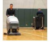
Mix WAXIE Ultra Prep (#320896) diluted at 8 ounces per gallon (1:16) of water into the autoscrubbers solution tank. WAXIE Ultra Prep will be applied to the floor surface while scrubbing. Always work the floor in the direction that the boards are going if possible, as this will help to insure that the proper overlapping of each pass is accomplished.
