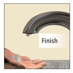
3. Soap is pulled back into the dispensing tube, reducing drips.
