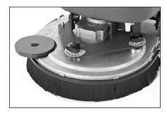
With the deck up, show how the pad driver/brush is removed by simply spinning it off by hand (counter-clockwise from above). A pad driver is shipped standard with the machine, and can be installed easily using the 'click-on' feature, by lowering the deck onto it and pressing the brush button (reference step 15).
