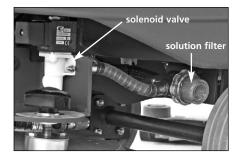
3 Show how the solution is gravity fed through the solution filter. The filter is easy to access and protected between the deck and machine. The solution flow is automatically turned on and off with the brush by means of a solenoid valve. The solution is shower fed through the center of the pad driver.
